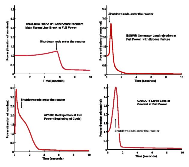
reactivity to -69 mk or more after 2 seconds. The peak total reactivity is +4.3 mk at 0.9 second (compared with the delayed neutron fraction of 5.2 mk) and the peak enthalpy is 638.5 J/g; Doppler feedback is small and negative. The total positive reactivity addition is about +15 mk at
